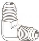
90° Union Elbow (Ref. SAE No. 070201) Assembly Number C35505x4, etc.
